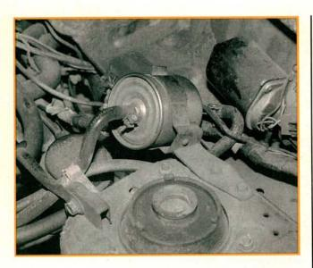
Suppose the car runs poorly, but there are no trouble codes. An external factor may be causing the problem. Low fuel pressure caused by a clogged fuel filter or other restriction may be forcing the ECU to keep the injectors open longer to compensate. This may show up as an abnormal Alpha reading, but the oxygen sensor reading may not indicate a lean mixture. Keep records. After practice with the same type of car, you will be able to identify normal and abnormal serial data readings.
