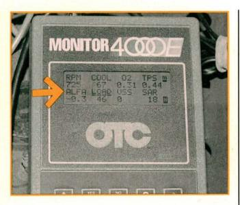
Two important data stream readings indicate the ECU's response to its sensor inputs. Alpha readings reflects the ECU's efforts to control the air/fuel ratio and are based on oxygen sensor signals to the ECU. Alpha readings are expressed as positive or negative percentages. Readings above zero indicate the air/fuel ratio is trending toward a rich mixture. The ECU will lean the mixture until Alpha reaches zero. The opposite process occurs when the Alpha reading is negative.
