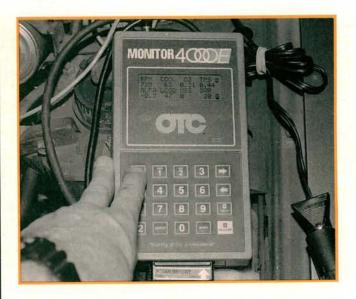
Custom Display allows viewing of up to eight different data stream readings at the same time. The selection and placement of the eight data items can be changed to suit the problem being diagnosed. A wider range of data can also be selected to find intermittent problems. The scanner update rate for some sensors is slower than a DVOM reading taken directly from the wiring harness. With practice, you'll recognize abnormal data stream readings before the ECU has a chance to signal a trouble code.
