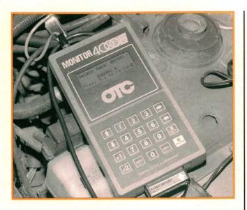
Subaru dealer technicians use a dedicated scanner called a Select Monitor to retrieve data from the engine management, cruise control, automatic climate control, and air suspension systems. We'll be using the OTC Monitor 4000E. One cartridge lets the Monitor handle the engine management systems on ten different Japanese and Korean vehicle lines, as well as automatic transmission tests on some Toyota models. After hook up, we run through a short procedure to acquaint the scanner with our Subaru.
