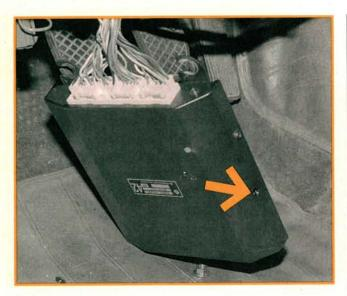
Japanese cars consisted of a Check Engine light. When the light came on, you knew there was a problem. The ECU might also include one or more diagnostic LEDs to retrieve trouble codes and measure oxygen sensor activity (arrow). Technicians with domestic car experience considered this absolutely primitive. But engine management system problems were few, and import technicians seldom missed the serial data diagnostics the domestic guys took for granted.
