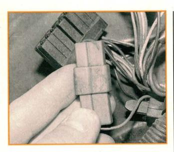
The Subaru system has four separate diagnostic modes (U-Check, Read Memory, D-Check, and Clear Memory). The ECU can be run through the different modes by either connecting or disconnecting the Read Memory and Test Mode connectors. We uncover our first glitch on this 1989 GL while running through the modes. The Check Engine light won't light, although the bulb and wiring are good. The engine seems to run normally, but the ECU can't call for help if a problem does exist.
