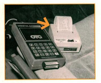
Intermittent problems may not show up while the car is sitting in the service bay. Using the extension cable, we can watch the scanner while an assistant drives the car. Customize the scanner to display the data stream information related to the problem. A portable printer (arrow) gives a written record of 13 different data items. Back at the shop, compare your readings to known good readings taken under similar driving conditions with a properly operating vehicle of the same type.
