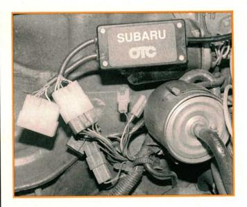
A scanner will give us a more complete look at the engine management system. Until standardized diagnostic connectors and locations become a reality, we'll have to deal with an assortment of jumper harnesses to adapt the scanner to different vehicles. Our Subaru diagnostic connector is located near the brake master cylinder, right next to the Test Mode and Read Memory connectors. Attach the scanner leads to the battery terminals for an uninterrupted power supply to the scanner.
