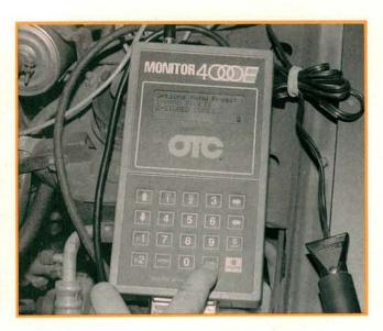
The ECU will set a trouble code if the sensor data it receives goes outside the limits that are programmed into the ECU's memory. The engine is running normally, but we'll check for stored codes just in case. Reading the scanner is faster than counting the LED flashes on the ECU. Two types of code storage are available. Hard codes signal a problem that exists right now. Stored codes are intermittent problems that cause a code number to be stored, but may not exist now. We have a clean slate.
