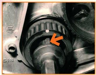
If you suspect that the crankshaft sprocket key has broken, the only way to check it is to remove the crankshaft timing sprocket. The sprocket may seem to fit tightly on the crank, and may lead you to believe that the key is okay. Remove the sprocket, then replace both crankshaft keys and the crankshaft seal.
