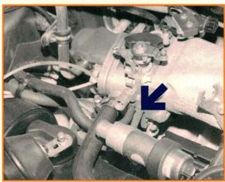
Don't assume that stuck fuel injectors are causing the problem. Remove the fuel pressure regulator vacuum line and check for fuel in the line. The vacuum line is attached to a vacuum port that's very near to the number 1 and 2 intake runners. Engine vacuum and fuel pressure force the fuel through the vacuum line from the leaking pressure regulator to the vacuum port. The extra fuel leaks into the intake manifold and causes number 1 and 2 cylinders to flood.
