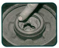
We removed both hub and rotor assemblies. New grease seals must have been hard to find the last time the bearings were repacked. The old, slightly distorted seals had been reused. At 78,000 miles, the condition of the wheel bearing grease indicated the bearings were long overdue for a repack.
