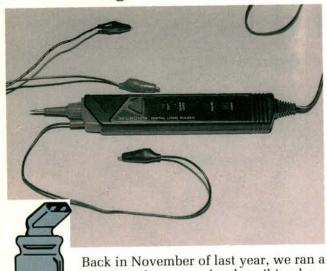
Back in November of last year, we ran a Tech Tip from a reader describing how to use a logic pulser (shown here) to trigger the injectors during fuel system testing. The logic pulser's square wave signal simulates the signals from the ECU to the injectors. We neglected to point out that the square wave signal emitted by most logic pulsers doesn't
