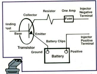
This simple wiring diagram describes the construction of the booster. A transistor from Radio Shack (P/N 276-2020) acts as a switching device for the ground supply to the injector. The 10 ohm 1 watt resistor acts as a dropping resistor to protect injectors that normally operate at lower voltages. The inline fuse protects the logic pulser in case the injector is
