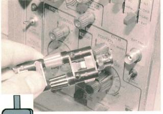
This is where Wayne's tip comes into play. We know we need an external trigger to "synch" our scope signal display, but how are we going to get the signal from the engine? An inductive RPM pickup is available for use with Fluke Automotive Meters. It can also be purchased separately. The RPM pickup has two banana plugs with standard spacing that are used to attach the pick-
