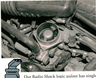
Our Radio Shack logic pulser has single and continuous modes. The single pulse mode doesn't last long enough to trigger the injector. In continuous mode, we could both hear and see the operation of the injector on this single point injection system. On multipoint systems, the logic pulser can be used to trigger individual injectors for a fuel delivery comparison.
