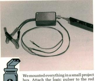
We mounted everything in a small project box. Attach the logic pulser to the red binding post at the end of the project box. Attach the heavy battery leads to the car battery, then locate the injector connectors in the wiring harness. We soldered micro alligator clips to the injector trigger power supply leads. Substitute a Bosch style harness
