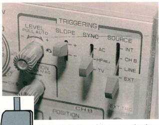
Fortunately, most lab scopes also have an external input terminal that can be used to synchronize the lab scope display. The signal information from the external input isn't displayed on the screen like the A and B channel inputs are. Instead, the scope uses the external input signal to decide "when" to display the signals from the other two channels.
