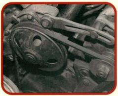
Leaking water pumps are a prime cause of head gasket failure. The engine cooling system design doesn't tolerate any fluid loss before it starts pumping air instead of coolant. No cabin heat, and a temp gauge that bobs up and down like a yo-yo are good signs that trouble is brewing—so to speak.
