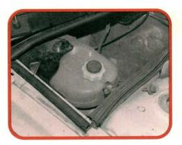
Later style cars placed the coolant jug in the water tray higher than the water pump, and the system was supposed to be self bleeding. A large lower hose from the jug fed coolant to the engine, and a smaller hose from the bleeding tee entered the top of the jug. This car has a blown head gasket anyhow.
