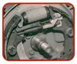
Another common problem was abnormal rear brake wear. We saw many cars arrive with uneven wear on the rear shoes. In some cases, one side had no lining left, while the other wheel looked like new. We eventually traced the problem to improperly adjusted hand brake cables.
