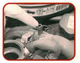
Add coolant until the remote fill neck is full. Then remove the short coolant hose to the bleed valve. What we're doing in this bleeding process is forcing any remaining trapped air in the cooling system to the highest point in the cooling system. Trapped air and this system just don't get along.
