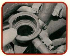
There's a lot of air trapped in the hoses above the radiator at this point, even though the radiator is full. Replace the radiator cap and remove the pressure cap at the remote fill neck. The remote fill neck is located on the right inner strut tower, right across from the water pump.
