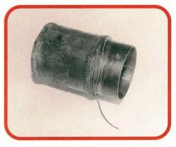
Renault used a single o-ring at the cylinder base to seal the cooling jacket from the crankcase. This made cylinder head removal a little tricky. If the head was unbolted and pulled straight up, the cylinders would stick to the head gasket and come along for the ride—breaking the seals.
