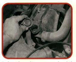
Early style cooling systems placed the coolant jug down low in the right inner fender. To fill this system from scratch, remove the radiator cap and fill the radiator. Be careful when removing the radiator caps. The plastic tanks get brittle from heat and the fill necks sometimes twist off with the cap.
