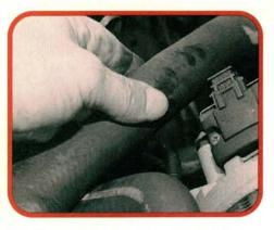
Set the cabin heat to HOT. Start squeezing and releasing the upper radiator hose. The thermostat is in the hose, and this process will fill the upper hose, purging most of the air from the upper hose through the thermostat jiggle valve. Make sure the thermostat's jiggle valve is at 12 o'clock!
