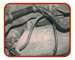
With the head removed, we get a better look at the vacuum hoses. On this car, one hose goes to the vacuum can, the other to the map sensor. These hoses cause all sorts of problems when they harden and crack from heat. Always check them and don't hesitate to replace them if they're suspect.
