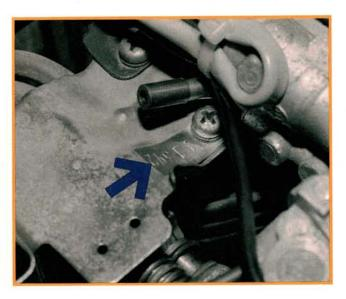
The carburetor must be replaced on some Tercels. Check the carburetor tag on top of the carburetor (arrow). If the five digit number on the tag is anything other than 11392 and 11402 (Federal models) or 11422 and 11432 (California models), the kit by itself won't help. Unless your customer has very deep pockets, you may want to stop right here. Replacing some of these carburetors also requires the replacement of a temperature switch and the addition of an engine compartment sub wiring harness.
