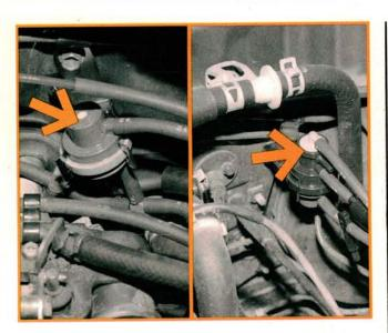
The two Vacuum Control Valve assemblies and vacuum hoses are preassembled. We'll refer to them as VCV-1 and VCV-2. VCV-1 can be identified by the open ended metal vacuum tee that points toward the VCV. Install the flat VCV-1 mounting bracket behind the carburetor, using the brake line mounting bolt. Install the offset VCV-2 mounting bracket near the brake booster, also using a brake line mounting bolt. Snap both VCV assemblies in their mounting brackets.
