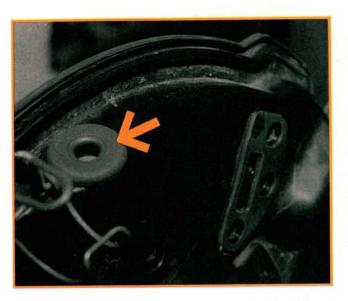
Remove the Electronic Bleed Control Valve (EBCV) from the air cleaner lower housing, then cover the filter housing air bleed holes with electrical tape. Clamp the housing in a vice, then mark the center of the area shown with a center punch. Use a 14 mm (9/16 in) hole saw to drill the housing, then install the grommet included in the kit. We'll pass the vacuum hose through the grommet to the accelerator pump air bleed later. Reinstall the EBCV and remove the electrical tape from the housing.
