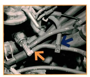
The VCV-2 needs a vacuum supply. Locate the yellow BVSV below the fuel pump (arrow). Disconnect the vacuum source hose from the BVSV's outer "L" port. Now route the vacuum hose from VCV-2 to the BVSB "L" port. The correct VCV-2 vacuum hose includes a yellow jet and an inline orange check valve. These are mounted in the VCV-2 hose between the intake manifold vacuum source and the vacuum tees we pointed out in the last step. Connect the intake manifold vacuum source hose to the black vacuum tee.
