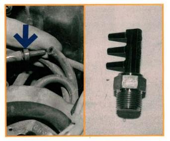
A couple more changes and our vacuum hose nightmare will be over. Manual transmission models need a purple jet installed in the vacuum modulator "R" port vacuum hose. We cut the hose about two inches from the modulator and installed the jet (left photo). We couldn't snag an on-car photo of the EGR BVSV (right photo). It's buried at the back of the intake manifold and must be replaced from underneath. Remove the air suction (AS) hose, AS reed valve, and intake manifold stay to reach the EGR BVSV.
