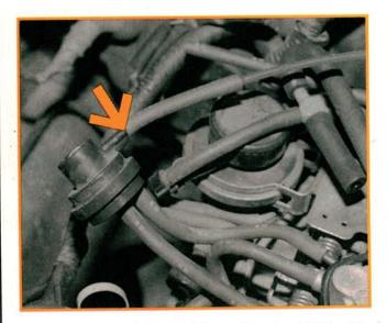
Locate the Choke Enrichment Breaker VCV next to the carburetor. Remove and discard the vacuum hose between the choke breaker VCV "S" port and the vacuum pipe near the carburetor. Cap the pipe with the vacuum plug included in the field fix kit. Swap the positions of the vacuum hoses leading to the choke breaker VCV "Z" and "Y" ports so the "S" port points toward the cowl. Now route the blue 330 mm hose from the open metal vacuum tee near VCV-1 to the choke breaker VCV "S" port.
