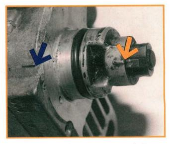
While the distributor was out, we repaired a common oil leak by replacing the distributor o-ring. Before installing the distributor, align the coupling groove with the notch on the distributor housing. Now align the second tab on the distributor flange with the valve cover bolt. The offset distributor shaft coupling prevents incorrect installation. Loosely install the distributor hold down bolts, then reinstall the plug wires, vacuum hoses, and harness connections.
