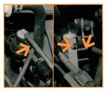
Route the other (330 mm) hose from the VCV-1 top hose tee across the engine compartment to the open "Z" port on VCV-2. Now route the insulated hose from the VCV-1 center "Z" port to the inside lower "L" port on the TVSV we installed in the water outlet housing. This hose can be identified by an air filter at the tee below the VCV. Route the other insulated hose from the VCV-1 "Y" port to the top "M" port of the TVSV. We'll route the last remaining hose to the carburetor air bleed tube later.
