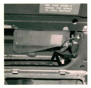
The ECU is mounted directly above the battery, behind the passenger compartment trim panel. Voltage drops shouldn't be a problem with such close mounting. However, mounting the ECU against an external body panel exposes
