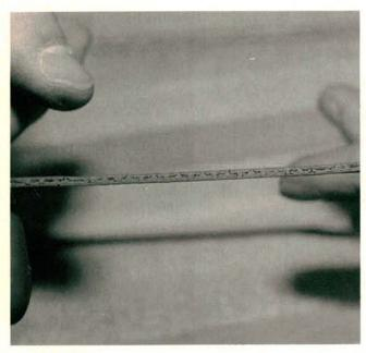
Leaking paper valve cover gaskets caused some engine fires on early Nissan Vans and resulted in the Van's first factory recall. The reinforcing material visible in this new style gasket prevents gasket splitting, and keeps the gasket in place under the valve cover.
