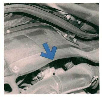
Remove the large metal reinforcing plate at the rear of the engine compartment (arrow) for extra room during valve cover removal or other maintenance work. To make more elbow room on the right side of the engine, remove the passenger seat and the large reinforcing plate that runs
