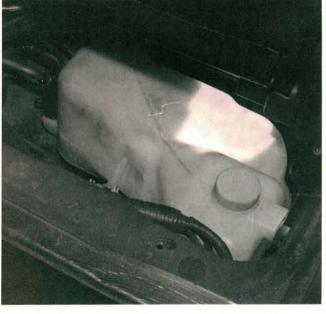
Move the passenger seat all the way forward, then remove the large metal access cover to service the coolant reservoir and fuel filter. Spilled fuel in this enclosed area is a fire risk. Relieve the fuel system pressure and clamp off the fuel line before changing the fuel filter.
