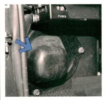
Replace the halogen headlight bulbs from inside the passenger compartment by removing the plastic covers (arrow). The fuse panel is tucked under the driver's side of the dash. Most electrical system relays are grouped along the right side of wiring diagram is a must for diagnosis.
