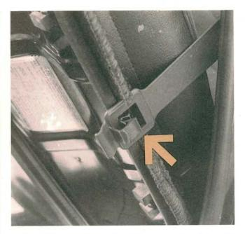
To raise the engine cover, slide the driver's seat all the way back so it will clear the steering wheel, then lift the front of the engine cover and driver's seat assembly. Tilt the cover rearward, then keep the cover open by attaching the plastic strap that's mounted to the shoulder belt bolt.
