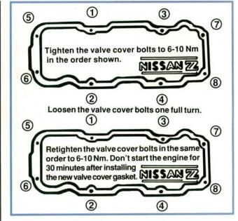
The valve cover bolt torquing procedures and torque specifications have also been revised. Use no sealer on the gasket and follow the procedure shown above. Factory part numbers have changed as the valve cover gasket design
