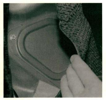
Turn back the carpeting to reach this small access plate behind the left rear corner of the passenger seat. Removing this plate gives you a view of the back side of the throttle housing. If you're double jointed, the automatic transmission dipstick can also be reached through this opening.
