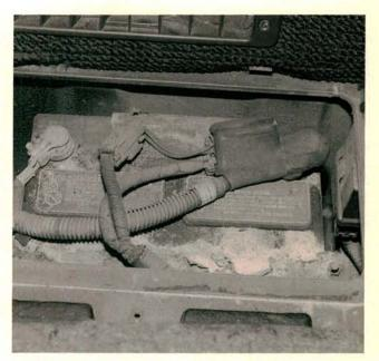
Locate the battery symbol on the left side of the rear passenger compartment, then remove the access plate under the carpeting to reach the battery. The battery tray is open to the elements from below. Clean the battery terminals and
