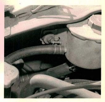
The most recent factory recall concentrated on the replacement of the cooling system and power steering hoses and other rubber parts. High heat loads under the engine cover put an extra strain on these parts. Always check hoses
