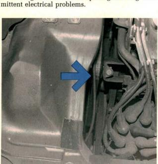
A failed radiator cooling fan clutch may cause a howling or squealing noise at temperatures below freezing on 1987-88 Vans. An updated cooling fan clutch was installed during the 90V-136 recall to increase airflow through the engine compartment and lower operating temperatures.
