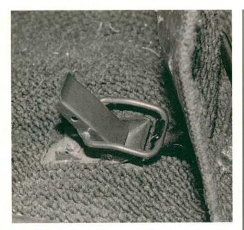
Just checking the oil level requires some work. Three latches under the carpeting keep the engine cover closed and keep the driver's seat firmly anchored in place. Two latches are located in front of the driver's seat, the third is near the left front corner of the passenger seat.
