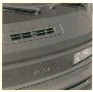
Unlike most front engine minivans, no maintenance other than headlight and wiper blade replacement can be performed from the front of the Van. Everything important must be serviced by working from either inside or below the vehicle. Adjust your labor estimates to reflect the
