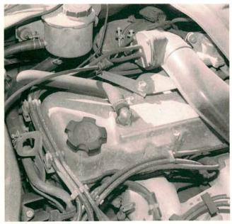
The Van's eight spark plug Z24 engine was used in Nissan pickups for many years. The biggest difference is that it's buried here. Engine oil and coolant can be added without much bother, but maintenance procedures like valve adjustments and spark plug changes require further
