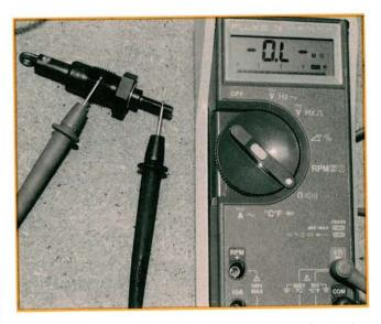
Next, clean all of the components with a wire wheel. That includes all resistor connectors, insulators, and the glow plug ends themselves. Then bench test every plug with an ohmmeter. At this point we're looking for shorts. Connect the ohmmeter leads between the body of the plug and the threaded contact as shown. If there's any continuity at all, replace the plug. Replace only those plugs that test bad.
