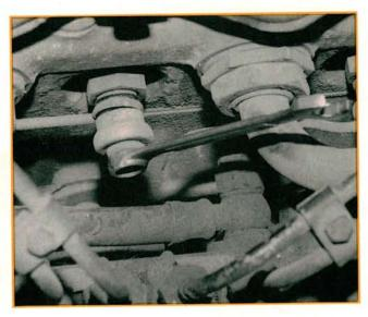
Using the same 8 mm wrench, begin removing the resistor loops from the plugs. Pay special attention to how they come off and also note their positions on the insulators. They must go back the same way they came off. Lay them aside in the order in which they're removed. Now remove all the glow plugs. Carbon build up in the head may make the glow plugs tough to remove, so don't be surprised if it takes some effort to unscrew them.
