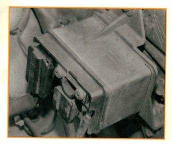
The glow relay is under the hood, on the left inner fender well. Remove the multipoint connector for the glow plug feeds, and test with an ohmmeter between each plug socket and engine ground. There is a numbering glitch on 1978-80 vehicles. The numbers on the relay terminal don't correspond to the respective glow plug number. We don't know why. Here are the match ups:
