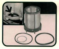
To prolong the automatic transmission life, change the fluid at least once every 30,000 miles or whenever it smells burnt. Remove these three bolts, then lower the cover to replace the round filter. The filter slides up into the transmission. Always use the new seals supplied with the new filter.
