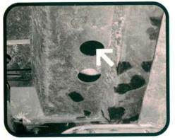
Look real hard and you might see the radiator drain plug in this photo. The plastic plug discourages overtightening but can also get brittle with age and may break if it's disturbed. To prevent an embarrassing leak a few days after a coolant flush, install a new drain plug or metal bolt.
