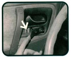
Removing the front door trim panel can give you fits if you don't know where all the hidden screws are located. Most of the screws are easy to find under plastic plugs. The last screw on the driver's side is behind the mirror switch. Pry the panel forward from the rear to remove it.
