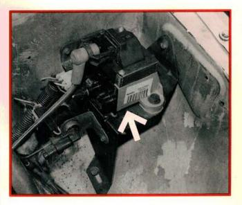
This combination Ignition Control Unit and conventional ignition coil receives the messages from the engine speed sensor. If you get a no-start, you'll probably test for secondary spark as an indication that the ICU is good. But that's not necessarily a foolproof test of the ICU. Use a noid light at the injector plug to test for injector triggers as you crank the engine. If you have secondary spark but no triggers, there's a good chance that the ICU is bad, even though you may have good spark.
