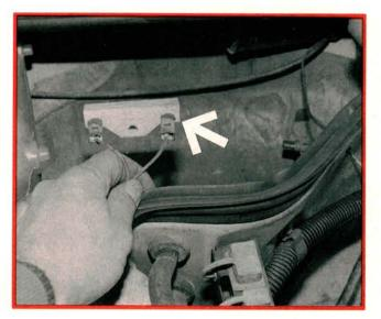
If an engine starts but stalls as soon as the key moves from the Crank to the Run position, check the ballast resistor for the fuel pump. It's located near the vacuum canister. The resistors themselves are pretty reliable, but as usual, the connections corrode. Clean and tighten the terminals and try again. The fuel pumps are inside the fuel tank. The fuel pump harness connector for some cars is located below the right rear quarter panel. Another good place to look for a bad connection.
