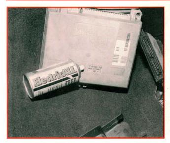
The ECUs were pretty dependable when they weren't being electrocuted or lethally injected with battery acid. Occasionally, when everything else checked out okay but the car still didn't run, we simply unplugged the ECU harness and sprayed all the contacts with contact cleaner. Many times, this fixed the car. The ECU is located under the dash on the passenger side of the car. If you do know someone with the MS1700 tester, the ECU can be removed from the car and tested separately.
