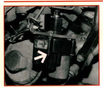
Actuator. Each time the engine is turned off, you should hear the ISA motor ratchet forward, click, and stop. This positions the throttle for the next start. These ISA motors do go bad, and we have also received several reports of poor connections at the plug going into the motor. The ISA bolts to the side of the throttle body. Be careful when removing the retainer nuts at the motor. The threaded studs can back out of the housing, leaving you with a handful of tiny plastic gears.
