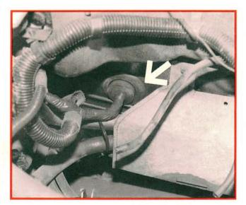
Early cars mounted the battery in the water tray on the right side. The factory batteries had removable caps. Water from a heavy rain or melting snow would run down the windshield and enter the battery through a not-quite-tight battery fill cap. The overfull batteries would spill electrolyte into the battery tray. In some cases, the acid would eat through the tray and run down the firewall to the ECU harness conveniently located below the battery. The acid followed the harness to the ECU.
