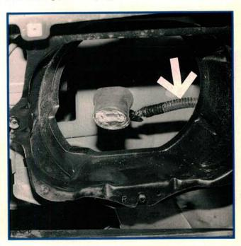
Raise the pop up headlights, then open up the protective outer wiring harness sheath below the headlights. Opening and closing the headlights hundreds of times eventually causes the wires to crack and break. Repair any damaged wiring, insulate the repair, then close up the wiring harness sheath. Route the headlight wiring harness so the headlights can open and close without pinching the wiring harness.
