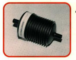
An inline filter can be added to the transmission cooler line for an extra measure of protection, especially on transmissions with inaccessible main filters. Some of these filters also include a magnet to trap metallic particles. Don't count on these filters to catch leftover particles from a sloppy rebuild, however.
