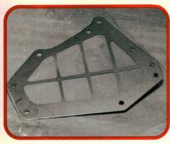
Some import transmission filters would make really nice screen doors. They do a great job of keeping large debris out of the transmission's inner workings, but often fall short when it comes to microscopic particles. Any dirt left from the last failure ends up here, eager to jam the valve body.
