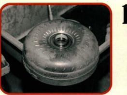
A torque converter can collect a lot of debris after a major transmission meltdown, and no amount of soaking and flushing the converter will remove all of the dirt. Maybe the customer's budget can't handle a new converter, but who's going to pick up the tab when your rebuild goes south?
