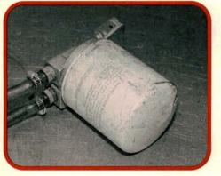
The transmission cooler is another hiding place for debris. Blowing out the cooler and lines doesn't mean you're safe. Installing this temporary auxiliary oil filter in the cooler lines catches any leftover debris during the rebuilt transmission's first several hours of operation.
