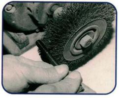
Check the threads on all reusable head bolts. Thoroughly clean the threads with a wire brush. Lightly lubricate the clean threads and the underside of each bolt head with engine oil before assembly. Dry, dirty, or damaged bolt threads can decrease the bolt's clamping force by as much as 50 percent.
