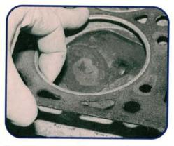
Carefully remove the old gasket. It can tell you a lot about previous engine problems. How the gasket separates from the mating surfaces may help you find where the failure occurred. Replacing the gasket without finding and correcting the reason for the original problem may cause the new gasket to fail prematurely.
