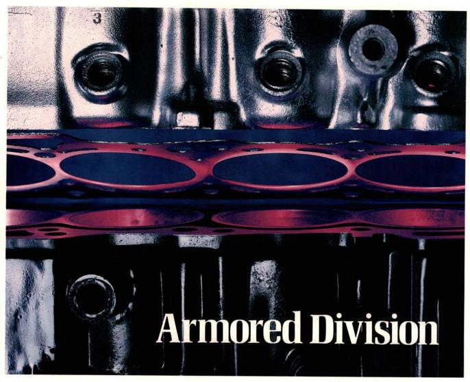
The head gasket serves as an armored division between the cylinder head and the engine block. This thin wafer of composite material maintains a state of relative peace and harmony between these two large chunks of often dissimilar metals.
