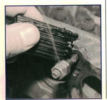
wax will be drawn into the threads, cleaning and lubricating them as it goes. Then after a turn or two with the wrench, the nut or bolt can usually be removed by hand (don't burn your fingers). This method also works well for removing a stubborn bearing collar.
