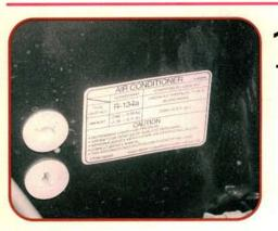
There are many differences between R-134a system components and their R-12 predecessors. To prevent accidental system cross connection and damage, all of these Nissan R-134a components are marked with a distinctive powder blue sticker. The main sticker lists lube type and charge quantities.
