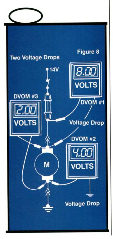
**Figure 8** shows a circuit which combines two of the first four circuit problems:
