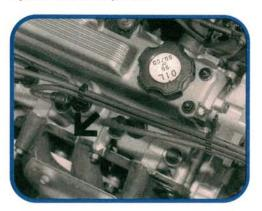
Early three cylinder Sprints (1985-86) may develop a coolant leak at the head gasket. Look for the leak at the front of the engine (in car position), in the area near the center cylinder. A revised head gasket was added to production to correct this problem and can be retrofitted to early models.
