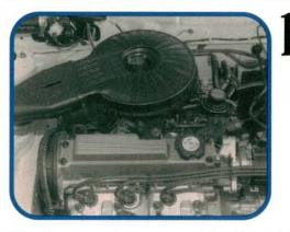
There's plenty of room to work in this engine compartment, thanks to the Sprint/Metro's three cylinder engine. The engine looks like it would be more at home sitting in a motorcycle frame. This engine requires periodic valve adjustments. Adjust the valves with the engine at operating temperature.
