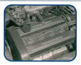
Suzuki saved a few extra fireworks for their own versions of these cars. Entry level Swifts are equipped with a single overhead cam four cylinder engine that also requires periodic valve adjustments. The Swift GT gets a twin cam four cylinder (shown here) with hydraulic lash adjusters.
