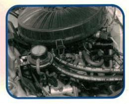
Sprints and Metros have had an assortment of fuel systems, including fuel injection with a turbo, throttle body injection, and a simple carburetor like the one on this base model Metro. We can't cover the adjustment procedures for each. Check a manual or the underhood sticker for the basic specifications.
