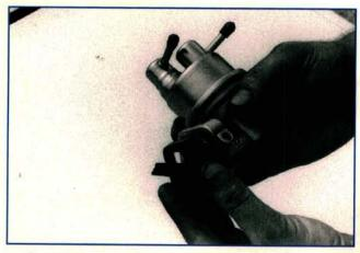
I have found this insulator to be a common source of oil leaks, either because it has cracked or the gaskets on either side have failed. I never replace a fuel pump without replacing the plastic insulator and its gaskets.
