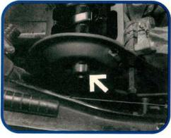
Tap on the back of the front cam sprocket to loosen it. Like the rear sprocket, it isn't keyed to the cam. But the front sprocket is different, and uses a tapered friction fit. Remove the bolt and sprocket, and pull the timing belt off to the side.
