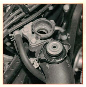
• Find an old radiator cap that is the same size as the one used on the cooling system you're working on. I only work on Nissans, so I only needed to round up a couple of old radiator caps.
