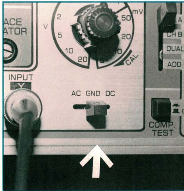
Location of the AC-DC-GND switch. Check the ground baseline and then switch back to the DC setting to make your tests.
