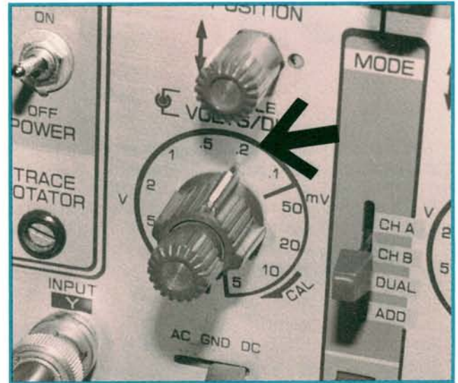
Setting the Volts/Div Knob to the 0.2 Volt setting.
