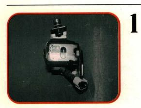
Supplemental restraint systems are most effective in front or front-angle collisions. The control unit must know the direction and strength of the impact so that it can decide whether the air bag(s) should be deployed. A series of sensors like this front crash zone sensor are used to gather this information.
