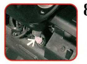
Most systems have connectors in the harness between the control module and the air bag module. If you must remove the module to center a steering wheel during a wheel alignment, separating one of these connectors (arrow) will reduce the possibility of an accidental air bag module deployment.
