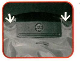
This air bag module was intentionally deployed during a test. The force of the expanding gases tore the outer module cover as the bag opened. Two large vents (arrows) allow the nylon mesh bag to start deflating as soon as it has filled. This cushions the impact as the driver hits the bag.
