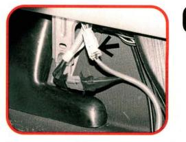
Every system we have seen uses a special harness connector color to identify SRS components and wiring. There's no mistaking the orange connectors in this Volvo SRS harness. However, this unprotected air bag module wiring easily could be damaged by a careless cellular phone installation.
