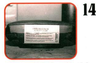
Always store a "live" air bag module with the outer cover facing upward as shown. If the module accidentally was deployed (an unlikely occurrence), this position allows room for the bag to harmlessly expand. If the cover is facing down, accidental deployment could turn the module into an unguided missile.
