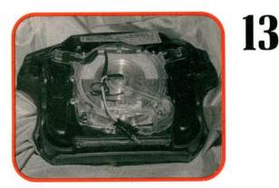
The air bag module is a sealed unit, so we can't show you the igniter squib and chemicals contained inside. A small amount of chemical dust is vented when the air bag is deployed. Use hand and eye protection when handling a deployed air bag module. These chemicals can cause skin and eye irritation.
