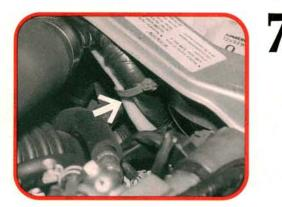
Nissan uses yellow SRS wiring harness connectors, and they also separate the SRS wiring harness from all other vehicle wiring and wrap it in a yellow plastic sleeve (arrow). Nissan allows no SRS wiring harness repairs. If any harness damage is found, the whole harness must be replaced.
