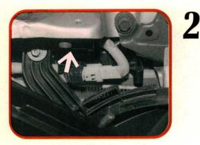
This Nissan 300 ZX has three crash zone sensors at the front of the vehicle. One sensor is mounted at each front corner, while the center crash sensor is mounted below the hood latch (arrow). The number and placement of these crash zone sensors will vary from vehicle to vehicle.
