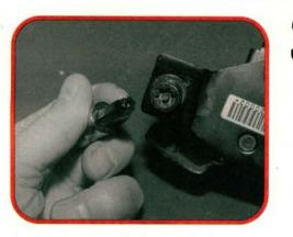
Anti-tamper Torx bolts attach the sensors to the body. A special hollow center Torx bit is required to engage the bolts. All bolts have locking compound applied to their threads and must not be reused if they are removed. The position indicator on the sensor assures proper sensor operation.
