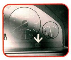
The SRS warning light informs the driver of system operation. If the system is working normally, the light should go out several seconds after the ignition is switched on. The warning light will stay on or flash to indicate a problem. This will also disable the system until the problem in corrected.
