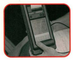
Nissan technicians can plug this dedicated CONSULT diagnostic unit into the main diagnostic connector for air bag diagnosis. The control unit has three self-diagnostic modes (USER MODE, PRESENT MODE, and INITIAL MODE.) to help determine if a fault is hard (PRESENT MODE), or intermittent (INITIAL MODE).
