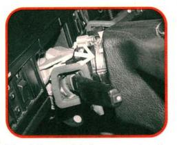
The air bag module is connected to the steering column wiring by a spiral cable mechanism (arrow). Unlike the simple slip rings used for steering wheel horn control wiring, the spiral cable maintains a reliable physical connection between the control unit and the air bag module at all times.
