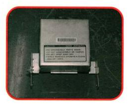
For an extra measure of sensitivity, this Nissan system includes a tunnel sensor and a safing sensor. Both sensors are contained in one unit. Before the control unit will deploy the air bag, it must receive a signal from at least one of the front crash sensors or the tunnel sensor, plus the safing sensor.
