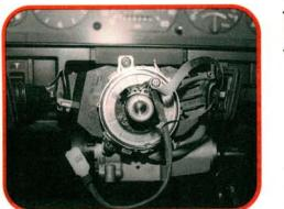
Spiral cable designs and locking procedures vary among manufacturers. Checking a manual before you try to yank the wheel will help avoid damage or extra work. If the wheel is removed without locking the spiral cable, the spiral cable must be centered before the steering wheel can be reinstalled.
