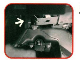
Some early SRS systems combine the control unit with a single, centrally located crash sensor. The Nissan control unit (arrow) receives all of its information from separate crash sensors, and is buried under the driver's side of the dash. The control unit can store nine different diagnostic codes.
