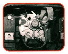
We've removed the air bag module in this photo. However, before we can remove the steering wheel, the spiral cable mechanism must be locked in place. On this Volvo, a special screw (arrow) is threaded into the spiral cable mechanism to lock it in place. The plastic ribbon explains the locking procedure.
