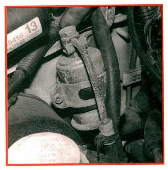
6 The oxygenated winter fuels used in some areas have been known to loosen fuel tank deposits. These deposits can work their way forward and clog the fuel filter, causing stalling or other driveability problems. Frequent fuel filter replacements may be necessary to prevent these problems.
