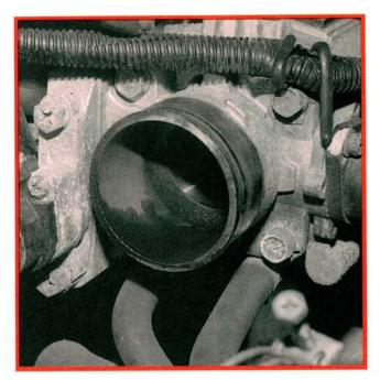
**10** Crankcase fumes and fuel deposits cause a build up on the inside of the throttle housing. If these deposits get thick enough, they can cause the throttle plate to stick or hang open slightly at idle. These deposits also throw off the throttle position sensor adjustment, causing driveability problems.
