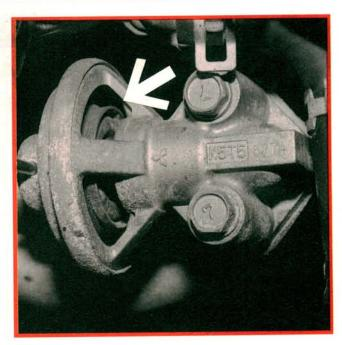
**8** The open design of the EGR valve may prove inviting to our four-legged friends. Unusual driveability problems may result when they leave nuts or other debris in the valve. Reach behind the intake manifold with your hand to check for a stuck EGR valve if diagnosing a rough idle condition.
