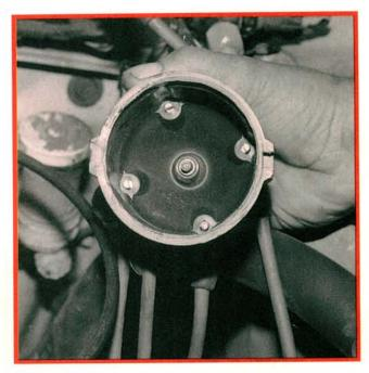
2 Flip the distributor cap over while you've got it off. Look for chalky deposits at the electrodes that can increase secondary resistance. On models equipped with a vacuum advance, check the unit with a vacuum pump. This is a common failure that may cause acceleration problems.
