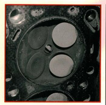
13 The owner of this DOHC engine decided to wait a few thousand more miles before replacing his timing belt. He made it all the way to 68,000 miles. The DOHC engines are valve benders, so this one clipped all eight exhaust valves, plus a few intakes. An expensive lesson in deferred maintenance.
