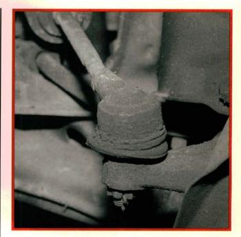
21 Mirages and Colts have a simple strut front suspension. Toe is the only adjustable front alignment angle. Service technicians tell us these vehicles normally hold an alignment for many miles. They watch for unusual tire wear or handling problems, then align problem vehicles when needed.
