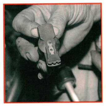
Electronic ignition can make you careless about secondary ignition components. High secondary resistance in other parts of the system may cause the secondary spark to burn holes through the distributor cap as it looks for an easier path to ground. Check for deposits on the tip of the rotor, too.
