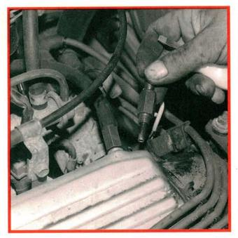
**9** The metal PCV valve threads into the valve cover. These valves should be replaced during a major maintenance to prevent crankcase ventilation and oil consumption problems. You probably won't be able to tell that the valve needs to be replaced by looking at it. When it's time, it's time.
