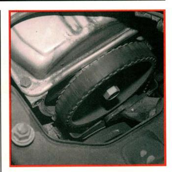
12 While you've got the upper cover off, check the timing belt for signs of wear and proper tension. Timing belt replacement is recommended at 60,000 mile intervals. Belts on SOHC engines usually make it to this interval without difficulty. The DOHC engines put more strain on the belt.
