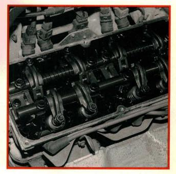
All single overhead cam engines require periodic valve adjustments. Adjustment on this two valve 1988 Mirage engine is normal. The smaller "jet" valve spring pressure on 1989 and later three valve engines is very light. The feeler gauge should slip past the valve stem with light resistance.
