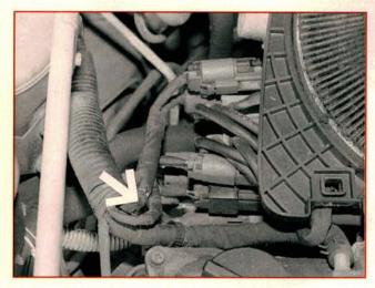
Check the ECU for stored trouble codes. If there are no codes, try pulling on the air flow meter wiring harness while the engine is running. If the engine dies while you're moving the wires, the orange wire in the air flow meter harness may be damaged. Open the wiring harness about three to four inches away from the connector and check for damaged wires. Repair the damaged wiring, then lengthen and re-route the harness to allow for normal engine movement.
