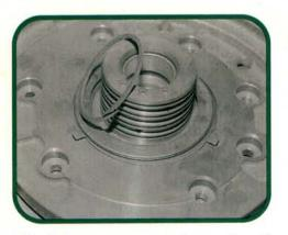
This brings us to some internal sealing problems which have resulted in failed 3/4 and reverse clutches. There are several possibilities to consider which may cause "cross-over" leaks between clutch fluid feed lines. Leaking seal rings on the pump are one possible cause of cross-over leaks.
