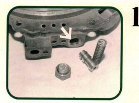
This is the early spool-type pressure control valve. It had a tendency to stick in the bore in the oil pump housing. The spring/piston assembly would stay open, causing erratic pump output pressures, even though the pump was just fine. A modified piston with a centering snout is available as a fix.
