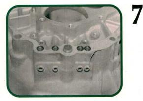
If you're splitting the case for any reason, always replace the o-rings between the case halves. Then seal the rest of the case halves with an approved sealer. This is one more place where cross-over leaks can occur. Don't let the cake decorator in the group apply the sealer. Excessive sealer can clog the ports.
