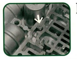
Those of you accustomed to seeing the pressure metering orifice holes in the valve body separator plates may find this wrinkle interesting. Tiny orifice cups on springs (arrow) have taken the place of precision drilled orifice holes in the separator. Don't lose, mix, or relocate these caps.
