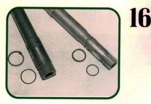
Another design change has to do with the input (turbine) shaft design. The early style shaft was meatier than the revised shaft. A Ford bulletin suggests that you always check the shafts for breakage, and replace the shaft and seals on any transaxle built before VIN#161020.
