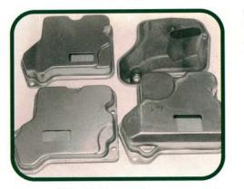
Filter and fluid changes became more important when they started using solenoids in valve bodies, so you'd better know the four filter options. Reading clockwise from top left: 1988-92 regular and turbo models; the new plastic-bodied filter used in 1993 versions; all hydraulic trannys; and 1986-87 versions.
