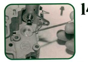
We mentioned plugged solenoids. The windings in the solenoids act as small electro-magnets, and attract any wandering metallic debris. When servicing or replacing solenoids, remove, clean, and reinstall the tiny filters in the bores where the solenoids fit and install new o-rings on the solenoids.
