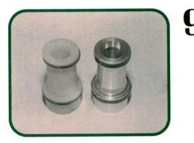
The original aluminum accumulator pistons were pretty, but they had a tendency to stick. You have two repair options here: either reuse the old pistons with new seals; or replace them with improved accumulator pistons and seals. We strongly suggest that you choose the latter option.
