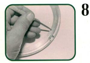
Cross-feed pressure problems caused reverse clutches to apply just far enough to drag when forward gears were selected. This caused overheating and premature reverse clutch failure. Some enterprising trans techs drilled a .030 hole in the reverse piston (pointer) to vent any cross-over pressure.
