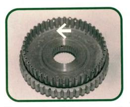
If you see a trans that won't move unless you select manual 1st or 2nd gear, suspect a bad input sprag. Be careful when you install a new one — it's possible to install it upside down. The sprag should freewheel in a counterclockwise direction (arrow) when it's properly installed.
