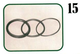
The 3/4 clutch piston inner seals can also cause confusion and an embarrassing comeback. This photo shows the different seal options, and a kit may contain all three. Choices include a lip seal and two o-rings. Use the wrong one, and you'll burn up the 3/4 clutch pack when it starts slipping.
