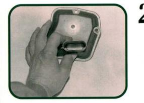
The filter used in 1993 versions incorporates an "American" style filtering element. Earlier versions used a screen-type filter we've seen on Japanese transmissions for years. But the screens weren't always fine enough to keep tiny bits of metallic debris out of the electro-magnetic solenoids.
