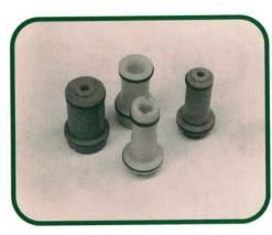
The valve body contains four separate accumulator pistons. These new, improved pistons come in four different designer colors! But be careful, the width of the scarf cut sealing rings for the plastic pistons is thinner than those used on the original aluminum pistons. Don't mix and match.
