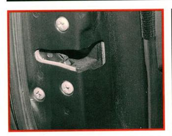
If the alarm system won't cancel when the driver's door is opened on 1985-88 Cressidas and Supras equipped with factory alarm systems, the most likely cause is a bad door latch switch. When you remove the door panel, there may be as many as four different kinds of door switches inside the door. They're all related to the alarm system. Before you pull out your hair, test the switch that is attached to the door latch mechanism. Experience has shown that this switch fails most often.
