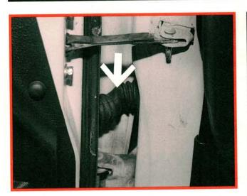
Dead radio speakers may be caused by broken wires inside the rubber door conduits. This problem seems to occur more frequently on the driver's side, probably because this door is opened and closed the most often. Peel open the rubber conduit, then check for broken wires. On vehicles equipped with power windows and power door locks, operation of these accessories may also be affected by broken wires inside the conduit.
