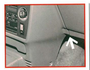
A failed temperature control motor may cause a no-heat complaint on Celica and Camry models equipped with automatic temperature control. The default position for the air mix door is full cold, so if the servo motor fails, the ATC can't control the temperature. To check the air mix door motor, reach under the dash while manipulating the heater controls. If the motor is working properly, you'll feel the motor move the door open and closed as the ATC is moved from full heat to full cold.
