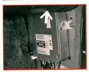
Water in the main relay may cause hard starting or a no-start condition on fuel injected Truck models. The main relay is located on the right kick panel, above the ECU. Water from a leaking windshield may find its way into the relay and possibly the ECU. This problem can be difficult to diagnose because the system may randomly lose fuel pressure, spark, or both. Remove the trim panel, then check the relay for water or corrosion damage. Make sure the leaking windshield gets fixed, too.
