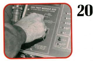
This is a four channel system, and has four solenoids to test—one for each wheel. By switching to each solenoid, we alternately test all of the valves by applying, releasing, and holding brake pressure. If any valve fails, either mechanically or electrically, the modulator fails.
