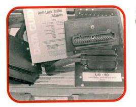
This breakout adapter from Thexton is one way to speed your tests. It provides an interface between many import and domestic ABS harnesses and a Ford 60 pin breakout box. Then use your Mitchell manual or comparable reference guide to determine correct pin numbers. **Thexton, Circle No. 140**.
