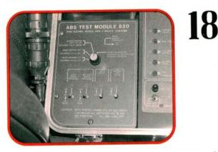
So how do you know when an ABS modulator is bad? We're about to use the 8400 tester to send a few signals of our own. We'll activate the control solenoids in each circuit to check proper operation of the modulator control valves in each of their three modes: Apply, Hold, and Release.
