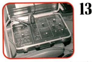
At a given vehicle speed, all wheel sensor inputs should be the same. A weak or missing signal can muddle the ABS control unit's mind. Today we're using the **AutoForce 8400 ABS tester (Circle No. 141)** to speed our tests, and also to give you a better mental image of common test procedures.
