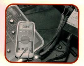
Erratic signals from any one sensor can indicate a problem. Maybe the sensor wheel is partially plugged with rust or debris, or has more teeth missing than an NHL goalie. We can measure peak voltage levels of each sensor by plugging a DVOM into the tester's breakout pins.
