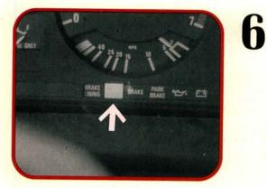
The ABS dash light should cycle through a normal bulb check sequence, and go out within a few seconds after starting the engine. If the bulb does not come on with the Key ON/Engine OFF, find out why. Some bulbs have been removed when other repair attempts failed. This deactivates the ABS.
