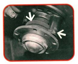
The most important inputs to the control unit are the speed sensor signals. The BMW's front sensors are mounted near a toothed ring on the wheel hub (left arrow), and are protected by a metal cover (right arrow). They transmit an A/C voltage signal to the control unit proportional to vehicle speed.
