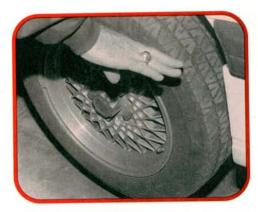
We're going to raise the vehicle, apply the brakes, and press the HOLD button after selecting a wheel. If the wiring to the actuator and the solenoids inside it are good, the brake should stay applied until we press the Release button. Do not perform these tests out on the road, for safety's sake.
