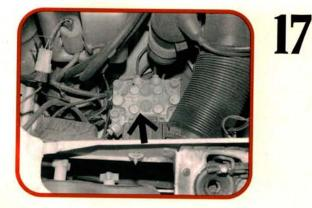
From all reports, ABS hydraulic modulators (arrow) are very reliable. Blame them only as a last resort. Any thoughts about servicing them in the field should be freely sprinkled with the word "liability" and permanently placed on the proverbial back burner. Replace a bad modulator with a new one.
