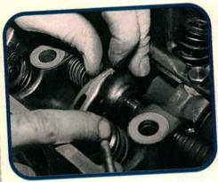
Turn the cam until most of the valves are closed. Push each rocker arm against its rocker shaft spring, then remove the rocker shaft spring clip with a pocket screwdriver. One side of the clip gets all the wear, due to contact with the thrust ring. Always replace these clips during an overhaul.
