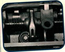
After loosening all of the rocker arm adjusters, two or three partially opened valves will prevent camshaft removal. A special BMW fixture is available to depress the valves, or screwdrivers may be used to open the valves. We chose to remove the rocker shafts first, then the camshaft.
