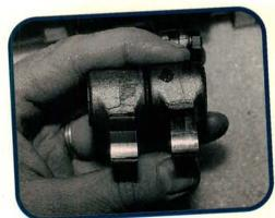
Given the extended oil change intervals we knew this engine had endured, we expected to find a set of rocker arms like the one on the left. It's actually a ringer from a different engine with a lot fewer miles. Poor quality follower slippers have been known to break off the aluminum rocker arm.
