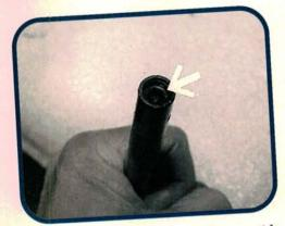
There are four rocker shafts, two per side. Each shaft is different, and can only be installed in one location in the head. Some shafts are tapped, with a hex head plug in one end (arrow). After removing the plug, a slide hammer adapter can be used to pull each rocker shaft out of the head.
