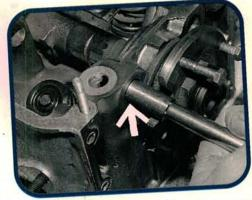
These rocker shafts aren't threaded, so we'll drive them out of the head instead. We used a modified socket and long socket extension to push out the rocker shafts. To avoid damaging the rocker shaft thrust rings, drive the rocker shafts from the end of the shaft facing the thrust rings.
