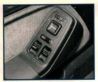
Erratic power window operation may be caused by a defective master switch in the driver's door. Because of the way the system is wired, operation of the window switches in all of the other doors can be affected by a messed up master switch. If the right rear window won't go up or down, check the motor by powering the motor directly. If the motor operates, the master switch is most likely to blame. Some switches can be disassembled and cleaned, but you may want to replace the switch to be safe.
