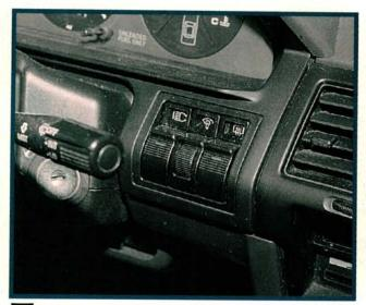
Battery discharge on 1986-89 Accord models may be caused by the rear window defogger. Driving at low speeds for extended periods with the defogger turned on may discharge the battery. A new defogger switch with a 25 minute timed cutoff (P/N 35500-SE0-A11) is available for 1986-87 models. A battery cover kit (P/N 06377-SE3-A00) to reduce the effects of high underhood temperatures is available for all 1986-89 models. Make sure the battery is fully charged before returning the car to the customer.
