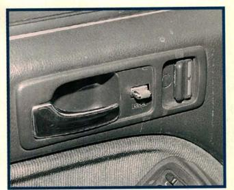
Smashed wires behind the driver's inner door handle plate may cause unusual power door lock symptoms on 1986-89 Accord models. After closing and locking all of the doors, one or more of the door lock actuators may make a clicking noise as they try to relock themselves. The phantom locks are caused by smashed wires or a defective actuator. Remove the driver's door panel, then reposition the wires so that they are clear of the door handle plate.
