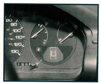
On 1990 Accord models, jump starting a discharged battery may affect the speedometer and tachometer operation. The low battery voltage, then sudden voltage surge may cause the speedometer and tach needles to rotate fully clockwise, then stay there. Do not replace the gauges to correct this problem. Use a small magnet to carefully rotate both gauge needles counterclockwise to their zero marks. Place a cloth over the magnet to avoid scratching the plastic gauge face.
