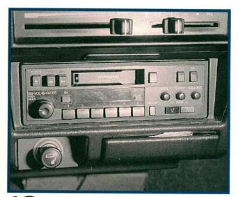
Intermittent radio problems are usually caused by poor harness connections at the back of the radio. If a speaker drops out intermittently, try tugging on the harness at the back of the radio to see if you can duplicate the symptoms. The harness is short, so you'll have to do this test with the radio installed. If the radio cuts out, remove the harness connectors to inspect for loose terminals. Giving male terminals a slight twist will ensure proper contact with the female terminals.
