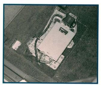
The engine and transmission control units are mounted on the floor and under the seats on many Honda models. The combination of this location and the recent flooding in the Midwest has put a lot of control units to the test. Trying to revive a wet control unit is a roll of the dice. You may be able to dry it out, but it may de-cide to act up later on. If you suspect that the control unit has been dunked at one time, open it up and look for light blue corrosion on the circuits.
