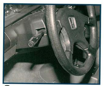
Headlight switches also wear out on high mileage Accords. This may cause the headlights to go out when hitting bumps (very exciting on a dark and rainy night). Try banging on the steering column with your hand or switching back and forth between high and low beams to see if the headlights will come back on. The one-piece combination switch that includes the headlights, turn signals, and wiper controls can't be disassembled for repairs and must be replaced as an assembly.
