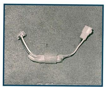
Intermittent operation of the blower fan control switch on 1986-87 Accord models equipped with A/C may be caused by the sub cord blower harness. This harness is located next to the blower motor assembly, and is equipped with what looks like a fuse holder. The fuse holder contains a diode, which may be causing the intermittent blower operation. The harness, which includes a female connector on one end and a male connector on the other for proper diode polarity, is available separately.
