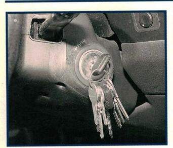
Worn ignition switches can cause intermittent electrical problems on all Honda models. Accessory operation (radio, heater, etc.) will usually be affected first, although some Civics may develop intermittent primary ignition problems caused by a worn ignition switch. Try wiggling the ignition key or banging on the steering column with the palm of your hand if you're having trouble duplicating an intermittent condition. Ignition switch replacement is the only permanent cure.
