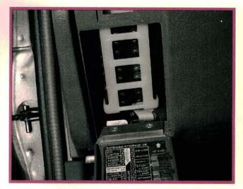
A quick check convinced us that plenty of spark was available. The healthy response to a whiff of carburetor cleaner down the throat of the air flow sensor seemed to confirm a decided lack of fuel. There was also an ominous silence from the fuel pump. We probed the blade-type fuel pump fuse with a test light and found power at both ends. So far, so good. But we wondered if this was destined to be the last sign of positive voltage we encountered.
