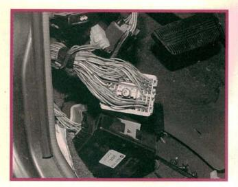
It is very important for you to make certain that you have the correct wires before taking the extreme measures mentioned in the previous caption. Several harnesses contain wires with identical colors, although their gauges may be different. Perhaps even more confusing, wires using the same colors in different combinations can also be found. For example, a red wire with a black stripe and a silver dash is NOT the same as a black wire with a red stripe and a silver dash. Check twice, cut once.
