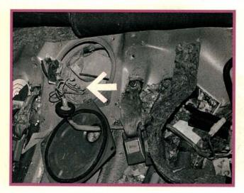
Previous experience with in-tank Maxima fuel pumps led us to pull up the back seat cushion to inspect the wiring at the top of the tank. The wagon's pump access cover is visible, but it can't be removed until you've also removed the eight rear seat back bolts. The tank top connections were okay, but Mummy's little helpers had scattered several funerary offerings in the area. The fuel pressure hose is barely visible. The stamped cover arrow must point forward to avoid wiring damage.
