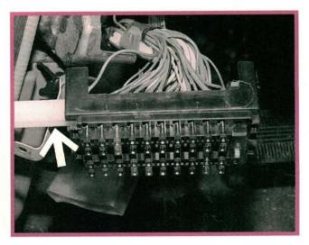
To replace the fuse-holder terminal, use a small screwdriver to remove the plastic retainer slide from the fuse panel. Then use your screwdriver again to release the locking tab that holds the terminal to the panel. The double terminal shown in the previous photo is suitable for the power input side of the fuse panel. You will need to separate one of the terminals at its base before it can be used on the panel's output side. Crimp and/or solder the terminal wiring, then reinstall it.
