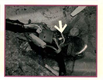
The multi-pin connector under the seat cushion was heavily corroded and stuck to the floor, apparently the victim of a soft drink spilled long ago. We replaced the male pin on the pump power feed wire when the old one came out in two pieces. Was this the break we had been waiting for? Unfortunately not, as the wire was still as dead as a second dynasty pharaoh. We wondered how the car had run in the first place. Was this a false start, or had we stumbled onto an ultimate cause?
