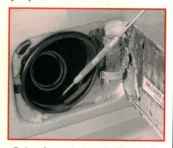
During a heavy rain storm, the filler neck boot can fill with water. The water has to go somewhere, and may find its way into the fuel tank.
