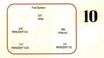
The four gas showed hydrocarbon, oxygen, and carbon monoxide levels were high, and the carbon dioxide level was low. Idle speed was also below normal. Removing the hose between the mass air flow sensor and the throttle body exposed some badly sludged throttle plates.
