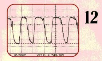
The  $O_2$  sensor waveform looked okay at 2500 RPM. The low voltage on the high end of the  $O_2$  sensor's oscillations (743.7 mV) concerned me, however. I like to see the sensor put out more than 800 mV at the top of its swing from lean to rich. I made a note of this abnormality and continued my diagnosis.
