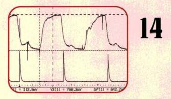
To figure out which cylinder was responsible for the misfires, I synced the  $O_2$  waveform with the ignition. The  $O_2$  sensor signal is definitely influenced by the cylinder firings. It is easy to measure the  $O_2$  response time, too. The rich/lean/rich transition times were well below 100 ms.
