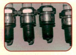
My spark plug inspection revealed worn center electrodes, but the plugs looked relatively clean. There was no indication of oil burning or abnormal combustion, just normal wear. The fuel filter also needed to be replaced, but the air filter was new. I noted these items on my estimate sheet.
