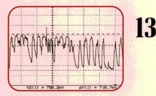
The  $O_2$  sensor's waveform looked terrible when the engine returned to idle. There were cylinder misfires (the sharp downward spikes seen in this waveform). The  $O_2$  signal should be independent of individual cylinder firings. This waveform isn't, indicating a misfire occurring in one cylinder.
