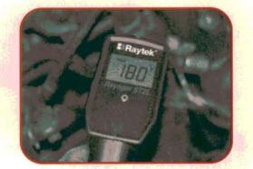
A new 180 degree thermostat brought the engine temperature and gauge up to par. You might not consider a thermostat replacement as part of a"tuneup," but a cold thermostat can cause a high idle, poor gas mileage, and excessive emissions. I had to replace it before continuing with the tune-up.
