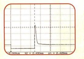
With new plugs installed, it was time for baseline measurements to determine the cause of the idle problem. The customer had declined any extra diagnostic time, but I still needed to focus on this area. The secondary ignition was fine and the injector pattern (shown here) was also normal.
