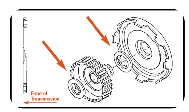
Also, when installing thrust bearing P/N 806537010, it is necessary to install two (2). One bearing is installed between the high clutch hub and the front sun gear, the other between the high clutch hub and high clutch drum. These bearings must be installed correctly. The smaller inner bearing race must face the front of the transmission.
