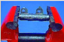
Compressing Belt Tensioner Piston
