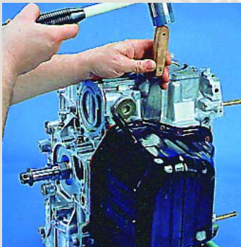
Removing Oil Pan
