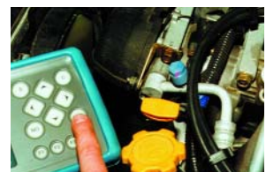
Figure 19 Monitoring A/C Relay Operation
