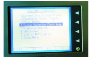
Figure 16 System Operation Check Mode
