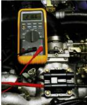
Figure 1 Measuring Secondary Resistance Between Terminals 1 and 2
