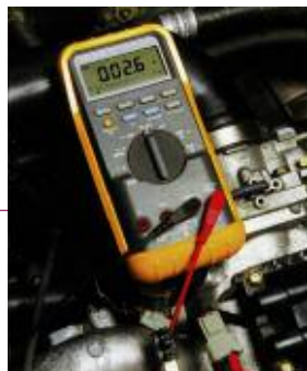
Figure 4 Measuring Primary Resistance Between Terminals 2 and 3
