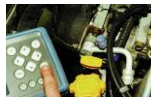
Figure 19 Monitoring A/C Relay Operation
