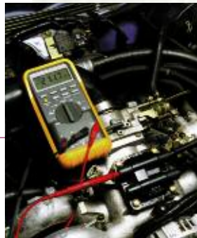
Figure 2 Measuring Secondary Resistance Between Terminals 3 and 4
