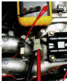
Figure 3 Measuring Primary Resistance Between Terminals 1 and 2
