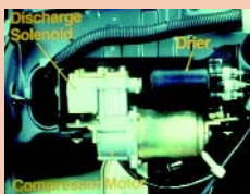
Air Suspension System Components
