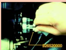
Air Pipe Remover
