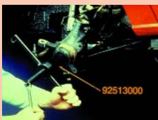
Replacing Drive Axle
