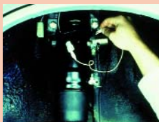
Venting Rear Air Spring
