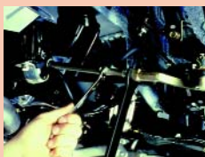
Front Toe Adjustment
