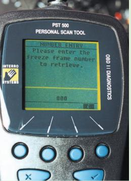
The PST500 interfaces with the vehicle ECU's via the standard J1962 OBD-II connector and performs the following operations:
