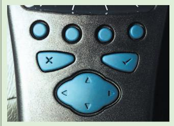
A single connection to the vehicle provides the PST500 with power and vehicle communications. Each time the PST500 is connected to a vehicle, it conducts a power-on self-test routine. All tool functions are handled by a 10-key silicone rubber keypad (shown).
