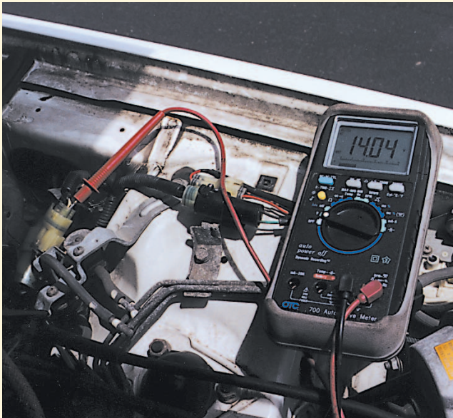
Above: Above 1800 rpm, voltage at the yellow/white wire to frequency solenoid valve B switches from zero to a pulsed battery voltage signal to control vacuum to air control valve B. Vacuum hose 17 vents to the air cleaner and hose 32. Hose 32 is also Teed into the upper chamber of air control valve B and to the white plastic vacuum regulator located to the right of the meter in this photo (it's behind the A/C idle up solenoid). Vacuum at the regulator is held to 5 in. hg.
