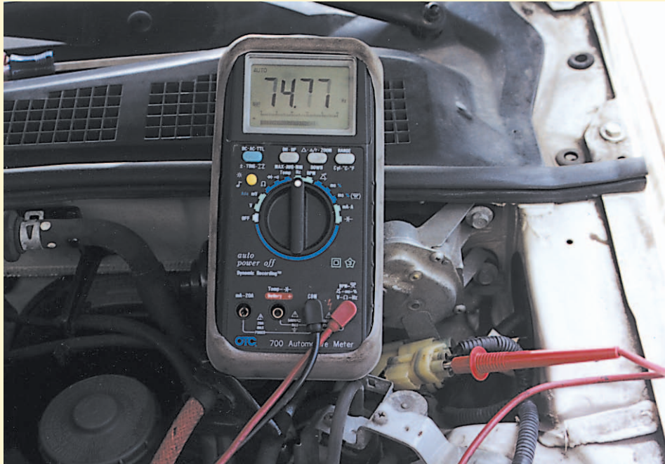
The yellow/white wire shows about 74 Hz with the meter set to frequency. The reading may normally fluctuate in a range between 40 and 80 Hz.
