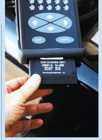
A separate data cartridge covers each carline. Slide the cartridge into place, noting the UP orientation. Attach the CS2000 battery connectors to power up the unit and begin initialization.
