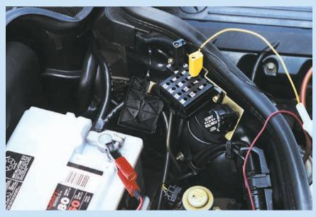
Based on your keypad selections, the CS2000 instructs you on the proper diagnostic terminals to insert the remaining diagnostic connectors. The procedures for Volkswagen and BMW are similar, although BMW utilizes a more convenient all-in-one diagnostic connector and matching CS2000 harness plug. Later M-B models also have this convenience.
