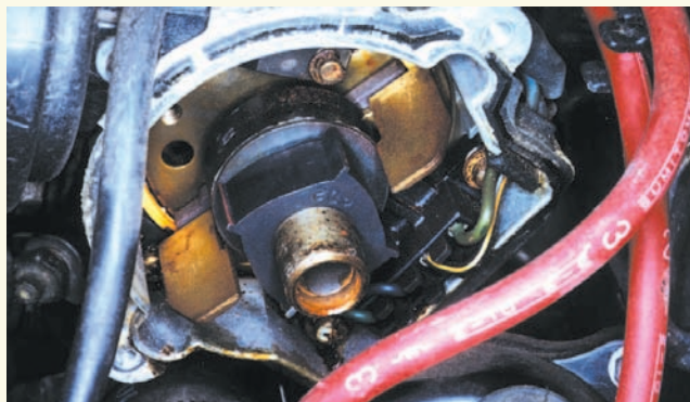
An early ignition distributor from an Integra, this unit contains only the cylinder position sensor, with the centrifugal and vacuum advance/retard diaphragms below and on one side.
