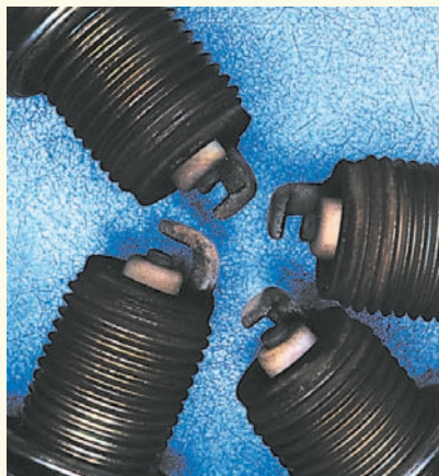
The whole purpose of the entire ignition system focuses on these gaps between the center and ground electrodes of the spark plugs. While newer, cleaner-burning cars can run a very long time on a set, plugs are not permanent parts of the car. The motorist has gotten his money's worth from this set.
