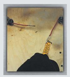
Our tests were nothing if not conclusive: In each case, the crimped connector held until the current melted the copper of the wire and broke the circuit open. In each contrasting case, the soldered connection melted before any of the copper wire burned. Looks like those Wolfsburg wizards did their homework on this one.
