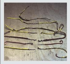
The pattern emerges: Each crimped connector held under the current load and mechanical tension until the wire melted; each soldered connection melted before the wire sustained damage. I guess VW was right.
