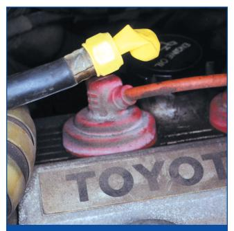
How to keep particulates and debris out of open air conditioner lines in the engine compartment? Be very careful, or swipe a kid's balloon and cover the exposed fitting with it.
