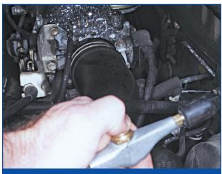
Foaming at the mouth? A soap solution over the suspect vacuum lines and shop air through the brake booster hose can often make the location of a vacuum leak conspicuous.
