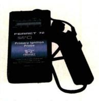
A BNC connector allows the user to view the waveform on most graphing multimeters or labscopes.
