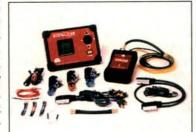
array of diagnostics, pinpointing specific problems in minutes. The operator can also choose from many individual tests to focus more clearly on aspects of interest. The tests include fuel pump voltage, system leakdown, an inductive test of the current draw and both static and dynamic injector flow tests. Besides those, it can also perform injector balance tests, volume tests and deadhead pressure measurements. Taking about five minutes to connect, its testing routine is completely automatic.
