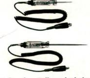
loaded strain relief is at the other. Bulbs on both the three-inch and the 6 1/2-inch probes are easily replaced.
