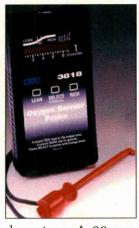
firm operation of the feedback system. A 20-segment bar graph indicates rich or lean, and the tool measures the activity level of the sensor to discover 'lazy' or inert sensors. An LCD display shows crosscounts. The tool works on a 9-volt battery, eliminating the need for power leads. It shuts itself off automatically.
