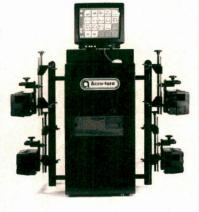
software and ALLDATA Undercar software. Four CCD headsallow quick and precise measurements of caster, camber and toe angles for all four wheels. A 17-inch monitor displays operating instructions, readings and three-dimensional adjustments. The system fits in a compact cabinet mounted on casters.
