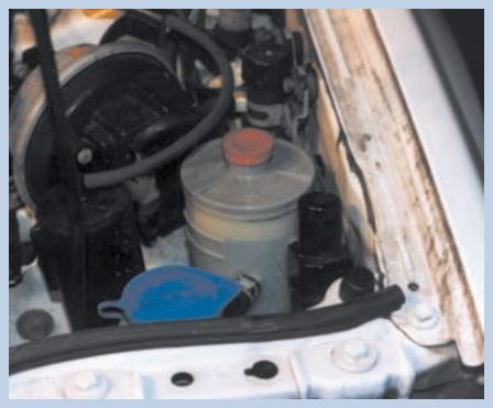
When you're sure you've got clean fluid throughout the system, reconnect the return line to the reservoir. Fill the reservoir to the upper line, then start the engine and turn the wheel back and forth as many times as necessary to purge air from the system. And finally top off the reservoir as necessary. It took a total of five bottles of power steering fluid to service this vehicle.
