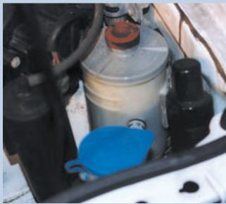
The fluid level on this Honda is just a bit low — even with the lower or "Min" level. Most of the time, we would make sure there weren't any leaks, then top off the reservoir with fluid designated "For Honda Power Steering Systems Only," right? Since Honda power steering fluid starts out clear like new engine oil and since the color of the fluid in this reservoir is dark, I opted to flush the system instead.
