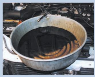
This is no exaggeration — the power steering fluid really was this dark. When you're done with the first evacuation of the system, fill the reservoir to the top with new fluid. Repeat the previous steps until clear fluid comes out the disconnected return line. Keep the reservoir filled so the pump always has as much new fluid as it needs.
