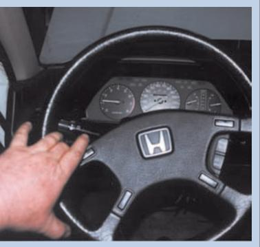
After hooking up the lines, start the engine. Turn the wheel all the way to the left, then all the way to the right as fast as you can, and shut the engine off. This allows the pump to push all the fluid out of the rack. Don't let the rack stop at full lock during this step. We're running all of the oil out of the system, and pumps don't like to run dry.
