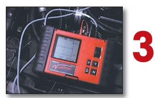
This is a peak power kV graph. The engine was running properly, so there's not much variation in the graph points. For example, high secondary resistance (an open plug wire) produces upward spikes. To isolate the problem, move the RPM probe to individual spark plug wires while viewing the measurements.
