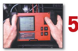
The tool's dual-screen capability allows simultaneous display of two secondary readings. On waste-spark systems, power and waste kV can be selected, for example. Or on a coil-on-plug system, you may wish to examine power kV and burn-time simultaneously. Readings may be stored for later study or printing.
