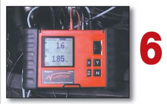
The dual screen capability can also display two readings in digital form. Here we simultaneously see digital spark kV and burntime readings. The Vantage has a five screen internal graph memory, and the Vantage PC Link software allows you to download stored graphs from the Vantage to a PC.
