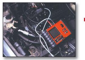
The dark gray RPM probe senses current in the spark plug wire you wish to trigger on. When triggered, a "T" is shown on the screen and you view measurements for the selected cylinder. If the "T" is not present, you are viewing measurements for all cylinders. The black capacitive probe clamps around the coil wire.
