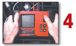
This is a spark kV graph, representing the voltage required to maintain the spark for the duration of the burn-time. Rather than looking for subtle changes in an oscilloscope secondary ignition waveform, the Vantage graphing capabilities allow you to identify abnormalities represented by high or low readings.
