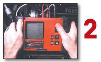
This doesn't look like a conventional oscilloscope ignition pattern, does it? The Vantage focuses on a specific section of the secondary ignition waveform, then presents it in histographic form. This graph represents burn-time. The graph should be uniform and between 1 and 3 milliseconds. If not, there's a problem.
