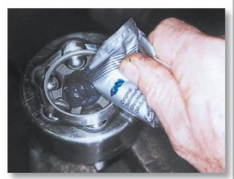
It wouldn't be a CV joint job without an envelope of special grease, squeezed, tamped and wiggled into all the passages of the balls and races. A new joint will be stiff when it's dry,  $but\ once\ you\ lubricate\ it,\ the\ shafts\ should\ move\ smoothly.$
