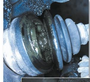
Both our Integra and Camry had the same problem, a split bellowsboot on the driver's side outer CV joint and just the beginnings of bearing wear. But we'd solve these identical problems in different ways.
