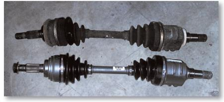
Once the Camry's shaft was out, we compared it carefully to the replacement. It's much easier to count splines and measure lengths and diameters on the floor or on the workbench than tangled under the suspension.
