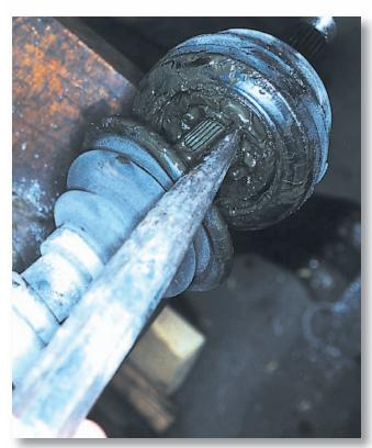
Since we were replacing the joint on the Integra, there was little reason to be particularly careful with the old internal races, tapping gently with a brass drift. Instead we just smacked it off quickly, being careful only of the splines on the shaft.
