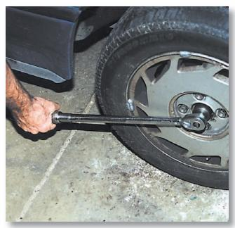
With the new shaft in the car and an assistant holding the wheel with the brake, tighten the axle nut to the shop manual's specifications. Don't guess and don't use an impact wrench for this job. Specifications vary considerably, and impact wrenches can destroy wheel bearings.
