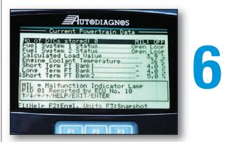
This screen should be familiar to all technicians. The Autodiagnos OBD-II pro cartridge displays OBD-II in its standardized form. The tester adjusts to reflect the characteristics of the selected vehicle's OBD-II system. Once again, the box at the bottom of the screen provides additional information on the selected item.
