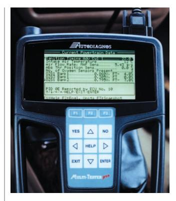
In addition to the Volvo serial interface capability, serial Volkswagen-Audi and OBD-II memory cartridges and harness connectors are available for the Multi-Tester *pro*. Cartridges and harness connectors for other major European brands (BMW, Mercedes-Benz) are also currently in development.
