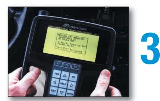
The Multi-Tester pro is collecting DTC's from the Brake/ABS control module. It's also possible to scan all available vehicle systems for stored DTC's. However, the pro didn't appear to know which systems the vehicle had until it checked for every possibility. Using the vehicle selection menu can avoid this.
