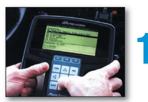
The Volkswagen-Audi memory cartridge is first. Early VW-Audi OBD systems use proprietary connectors, while later OBD-II compliant vehicles use the standard OBD-II connector to access their more extensive diagnostic capabilities. On-screen is a partial listing of potentially available vehicle systems.
