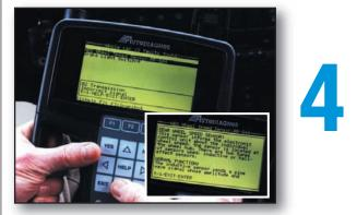
Two DTC's were detected during the whole-car scan. Highlighting an individual fault identifies the particular vehicle system (transmission in this example) gives additional information in the HELP box at the bottom of the screen. Pressing the F1 key provided additional information on the speed sensor (insert).
