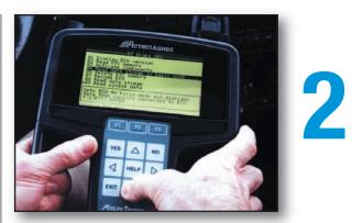
We selected the Brake/ABS system for further diagnosis. All choices for each vehicle system are arranged in a multiple choice menu format. The box below the menu choices provides additional information on the current menu selection. A separate HELP key provides additional information.
