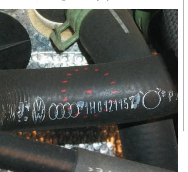
**5.** Here's how you can accurately test the thermostat opening setting. Many vehicles won't run in closed loop until the coolant temperature reaches a specific minimum. While thermostats are supposed to keep the engine warmer than that, with a noncontact thermometer, you can find out in precise, quantified detail. Measure directly at the thermostat housing or at the upper radiator hose on engines with more limited access.
