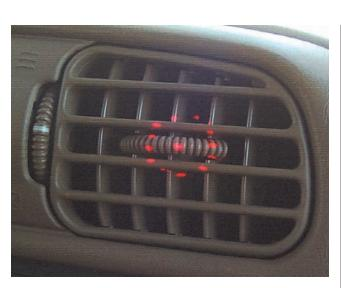
**7.** Check air temperatures at vents, heater and A/C outlets, more quickly and accurately than with a bimetallic-spring thermometer. In fact, since the surface of the duct is usually plastic and right in the path of the outrushing air, most frequently it will be at exactly the temperature of the heated or cooled air.
