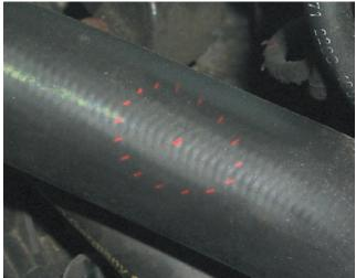
**6.** Check the temperature of the coolant as it goes back into the engine block. Is the engine overheating? There are half a dozen potential causes, but if the water going back into the engine is still warmer than it should be, there's a circulation block, a ram-air restriction or a radiator problem.
