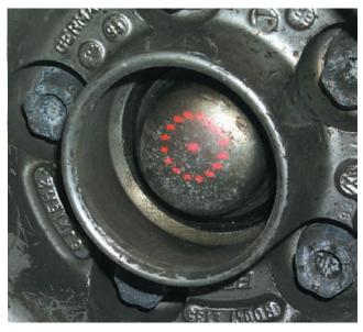
**13.** Friction in a wheel bearing will always generate heat. By the time you can hear noise as well, the bearing is not only worn out but even dangerous. Wheel bearings should ordinarily be just about at ambient temperatures unless heated by the brakes; if one is much warmer than its mate on the other side of the axle, something's amiss with that first bearing.
