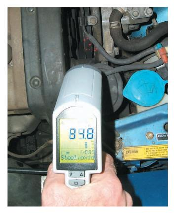
**15.** Are you hearing belt slip or wear in the bearings of the alternator or another accessory drive? Quicker than pulling most belts is just taking a quick thermal reading right after shutting down the engine. If the belt has been slipping, it should be considerably hotter than the surrounding material. If the problem was in a bearing, you may be able to locate that as well, given that the housing allows you a straight laser shot.
