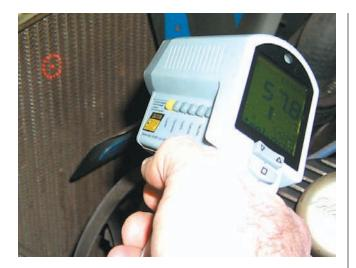
**3.** Find radiator problem locations. If several tubes in a radiator plug with deposits, you can find them using the noncontact thermometer over the surface of the radiator once the engine has grown warm enough to circulate the coolant. Radiator surface temperature should vary, of course, but there should be a smooth progression to the temperature change, not abrupt changes or pockets that stay at near-ambient conditions whatever else happens.
