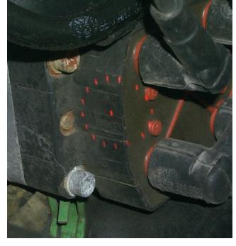
**9.** Check ignition modules and coils for unusually high temperatures. Darlington stacks in modules and power transistors of all kinds used as drivers produce a certain amount of heat naturally, requiring heat sinks, heat conductive grease and so on. If you cast an occasional diagnostic thermal spell over normal, functional units, however, you'll soon get a sense of what kinds of temperature might signal an imminent failure.
